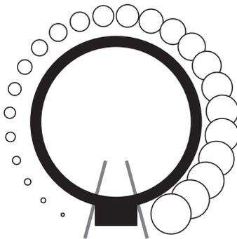
Use the rotary control to select any brightness level between 0.02 lumens and Maximum.
